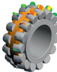
Spherical roller bearing showing progression of contact pressure and slippage
