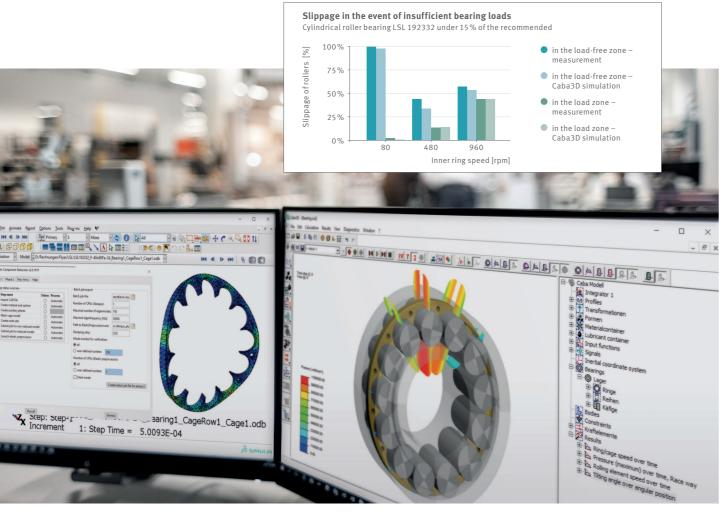
Caba3D is validated using tests and FEM calculations
