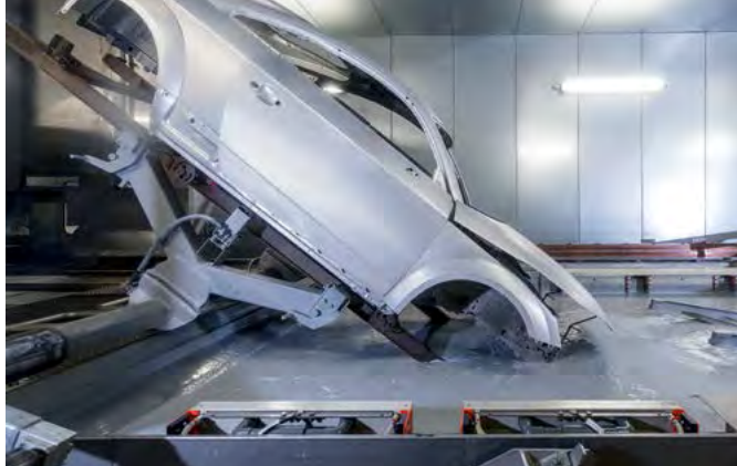
Dipped or sprayed: the coats are applied in various process steps
